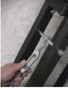
Hook the cable to cross barn near the end of the extension. Tighten the turn buckles to strengthen & straighten the Jib.
