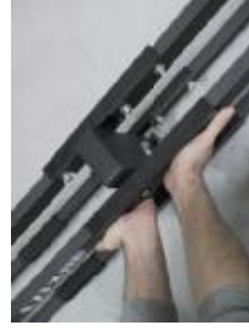
3. Connect an upper and a lower coupling channel to one side of the EZ FX Jib.
