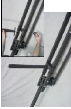
12. Attach the cable pole to the EZ FX Jib.
