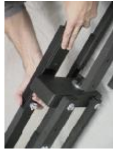
4. Attach the extension piece to the coupling channels.
