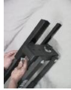
3. Connect an upper and a lower coupling channel to one side of the EZ FX Jib.
