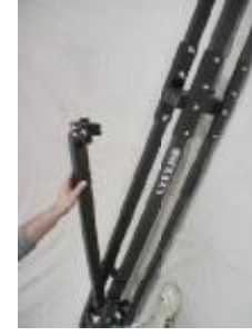
8. Fold over the tail arm of the jib to its extended position.
