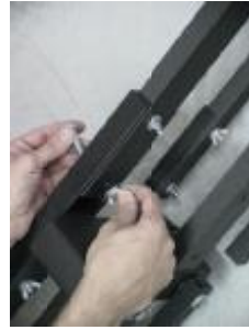
5. Use the bolts and wingnuts to secure the extension to the channels.
