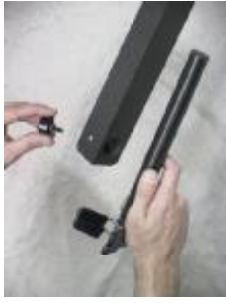
9. Remove the counter weight bar knob and longer 18" counter weight bar.
