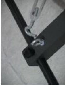
14. Hook the cable to the eyebolt at the end of the tail arm.
