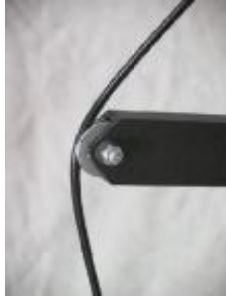
Run the cable over the roller at the top of the cable pole.
