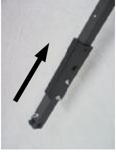
10. Loosen the wing nuts & slide the tail arm extension over the tail arm.
